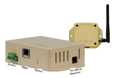
Spinwave Systems' BMS interface easily connects Spinwave's wireless sensors to open-protocol building automation systems.
